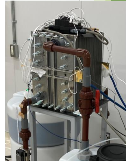
Product prototype cell stack 5 kW (442 cm 2 x 40 cells)
